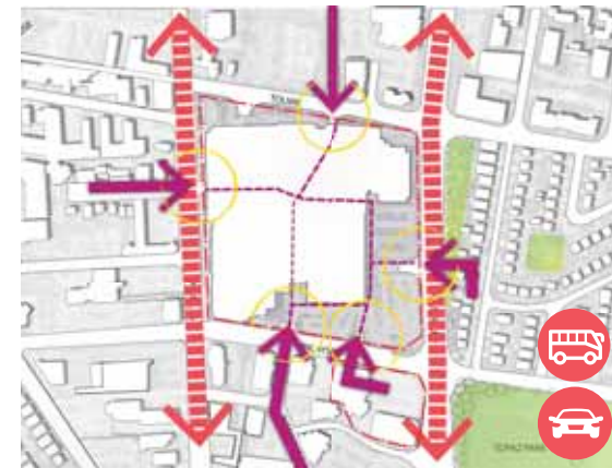
Vehicular access into and through the site is driven by adjacent streets' patterns, creating strong connections to the urban grid.
